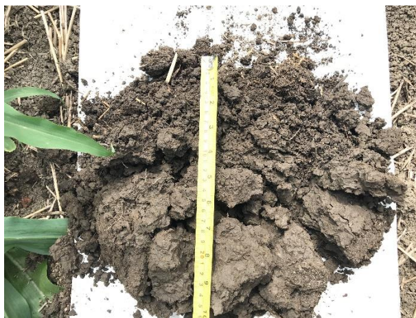
Figure 4. An example of a soil being evaluated using the visual evaluation of soil structure (VESS) within the soil structure assessment module.
